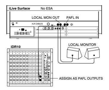
If you are not using Port A (EtherSound) to provide audio at the surface you can use analogue connections to route the PAFL signal from the MixRack to the Surface. Assign the PAFL mix to a pair of XLR sockets on the MixRack using the OUTPUTS screen. Plug XLR cables from the MixRack to the Surface PAFL in sockets. The PAFL signal now feeds the Surface headphones and local monitor system.
